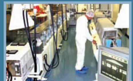
Watson-Marlow Pumpsil and Bioprene are manufactured in an ISO 14644 -1 Class 7 (Class J/10,000) clean room to guarantee no impurities
